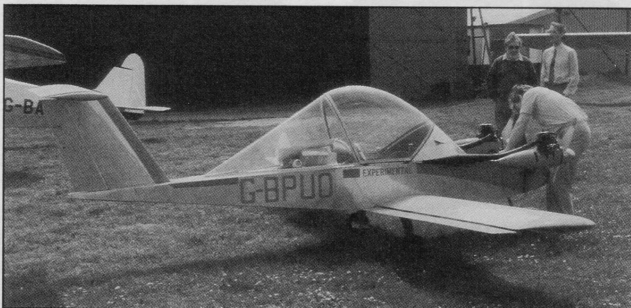
Low cross sectional area and streamlined "pilot fairing" give the Cri-Cri a remarkable performance on its 24 bhp. The high mounted "slab" tailplane has a bungee biasing system.
